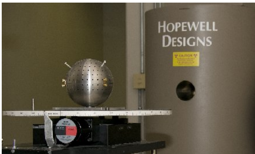
Figure 1: Photograph of RadBall Positioned in Front of an Automated Irradiator System at HPICL.
