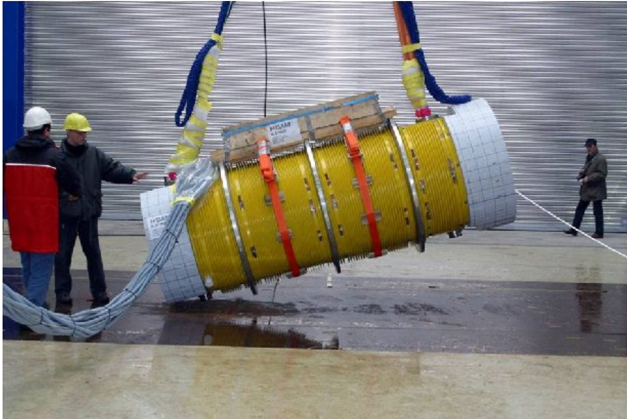
Fig. 6. 1:2 scale model CASTOR HAW/TB2
