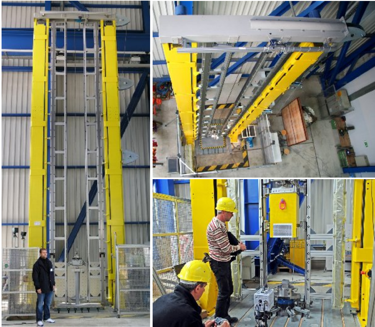
Fig. 7. 118-kJ Drop Test Machine
