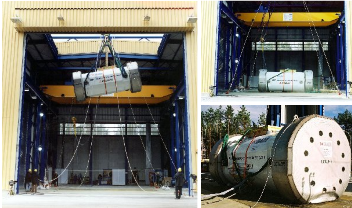
Fig. 5. 9 m slap-down drop test of the full-scale spent fuel cask design MSF-69BG
