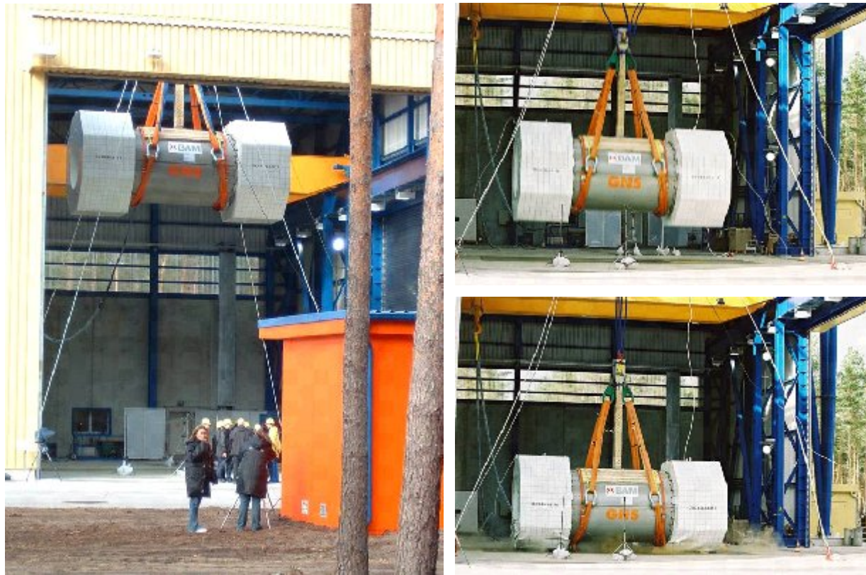
Fig. 4. 9 m horizontal drop test with the full-scale prototype of CONSTOR V/TC
