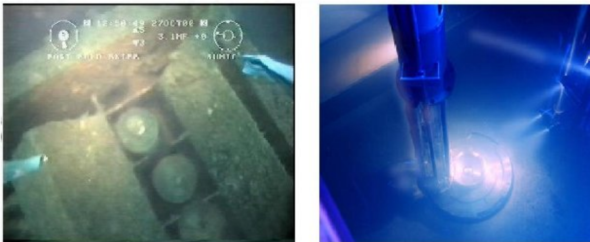
Fig.5. Canned fuel as stored in the pond and retrieval tool during works test
