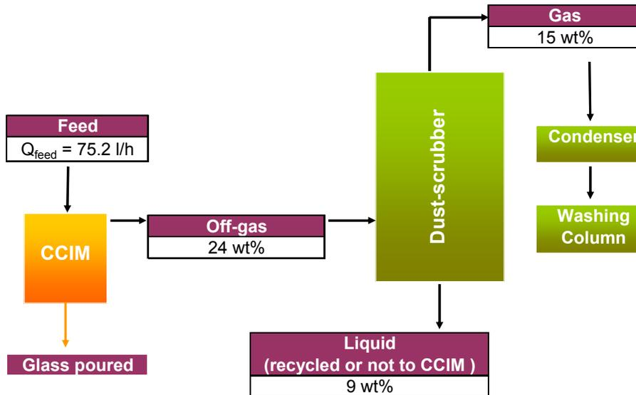
Fig. 3. Cesium Flow Sheet in weight percent, melter operated at 1,250°C, feed rate set at 75 L/hr (average values over 12 hours)
