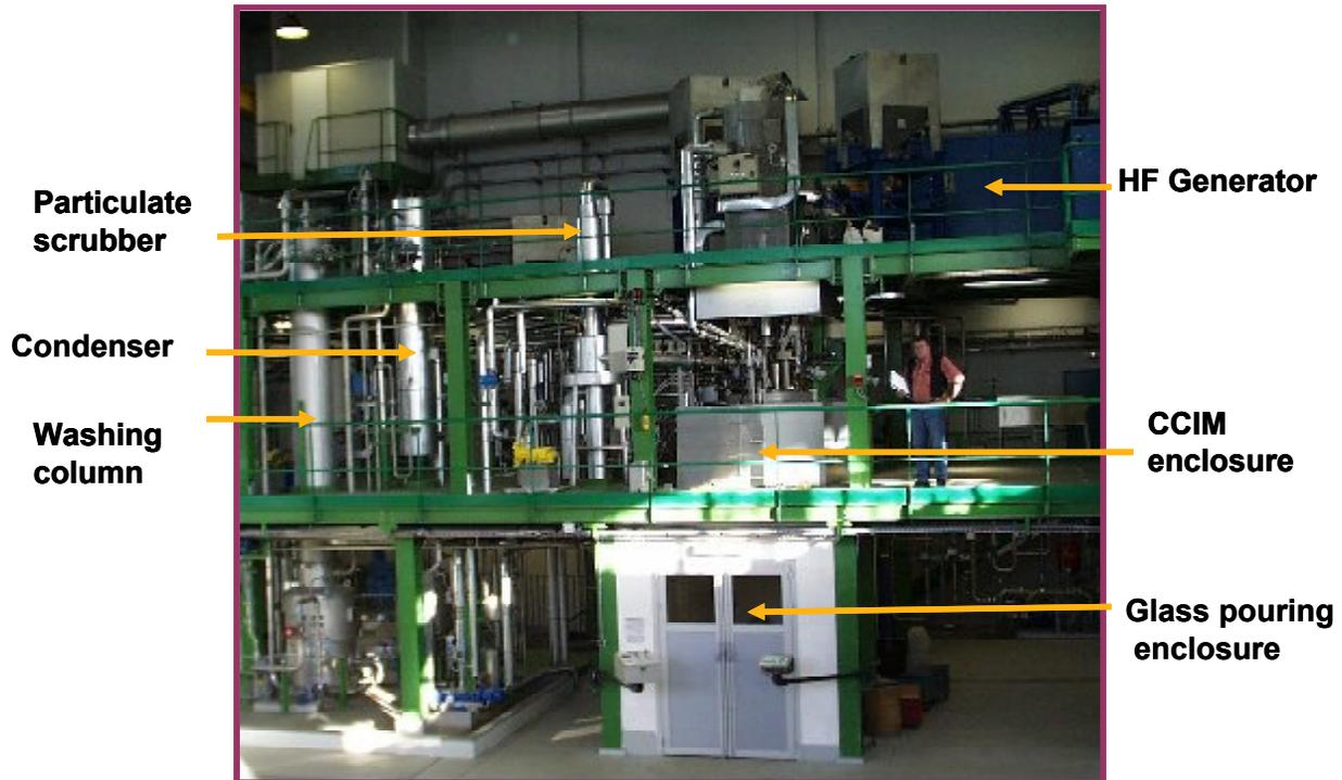
Fig.1: General View of the CCIM Demonstration Platform- CEA Marcoule
