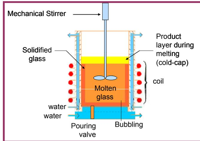
Fig.2: Basic Principles of the Cold Crucible Induction Melter
