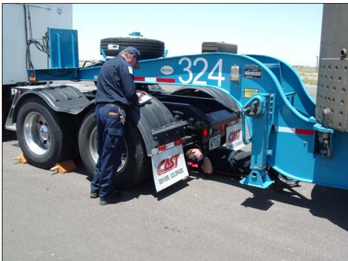
Fig. 2. A typical CVSA Level VI inspection being performed by Officers of the New Mexico State Motor Transportation Division of the New Mexico State Police
