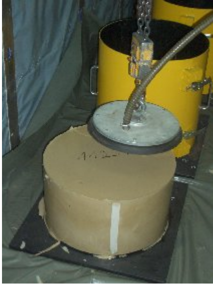
Fig. 7: Pellet coated with polyurethane
