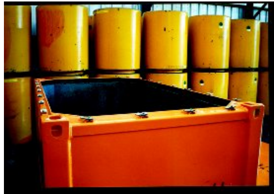
Fig. 9-9a: Old design of KONRAD container (lid not screwed on)
