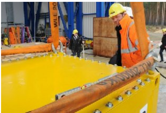
Fig. 10: New design of KONRAD container (lid screwed on)
