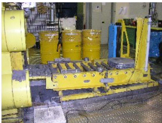
Fig. 6: Pressing in the supercompaction facility
