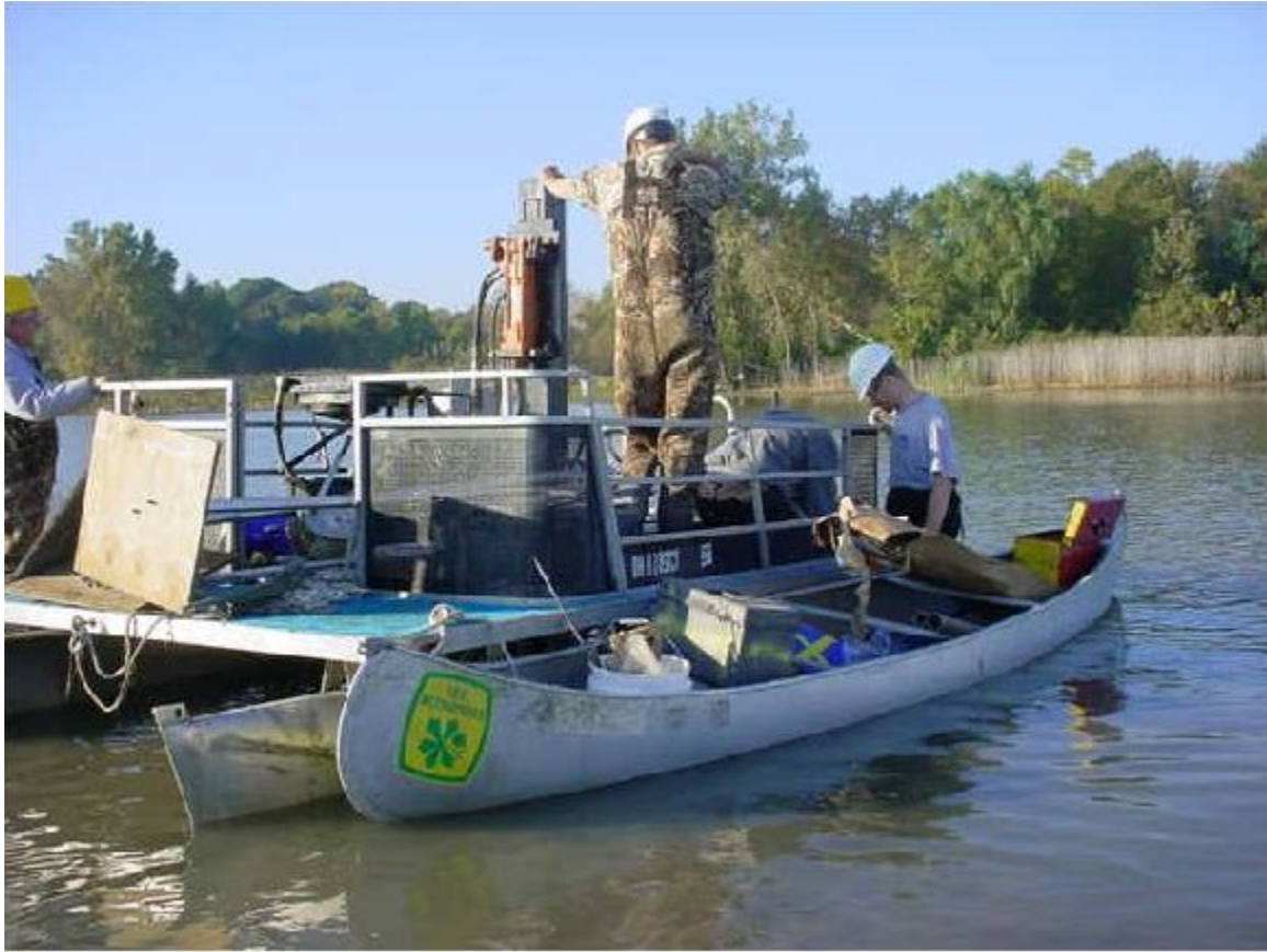
Fig 3. Pontoon Boat mounted geoprobe for sampling in Sandusky Bay
