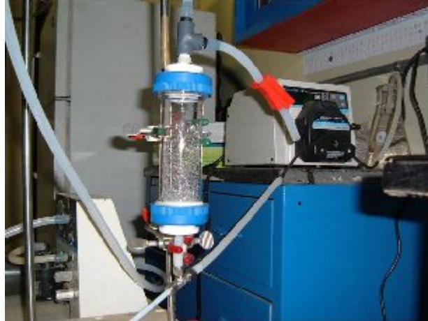
Fig 3. Porous plate foam generating apparatus.
