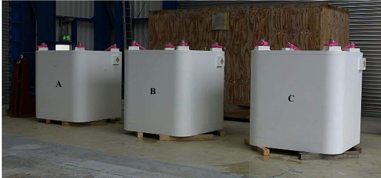
Figure.1. The three specimens A, B and C of the ‘Yoyushindo-Disposal’ waste container ready assembled for testing with different content masses inside the BAM drop test facility.
