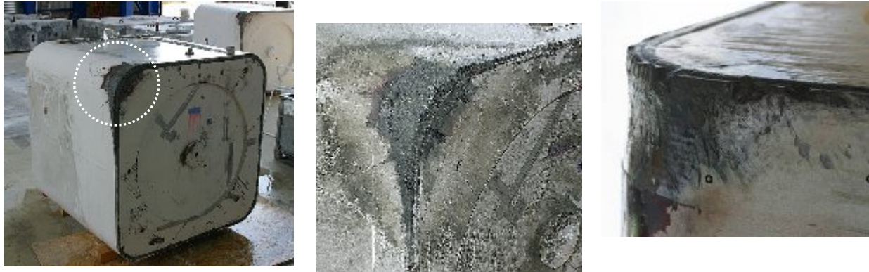
Figure 8. Specimen after drop test (left) with a detail photo of the impacted corner edge (right).
