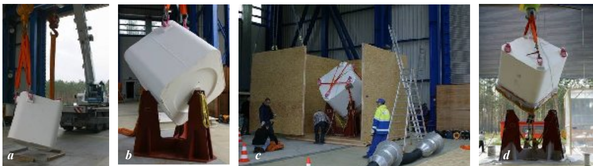
Figure 3: Cask handling (a, b: Pre-positioning, c: cooling, d: adjustment of exact drop orientation).
