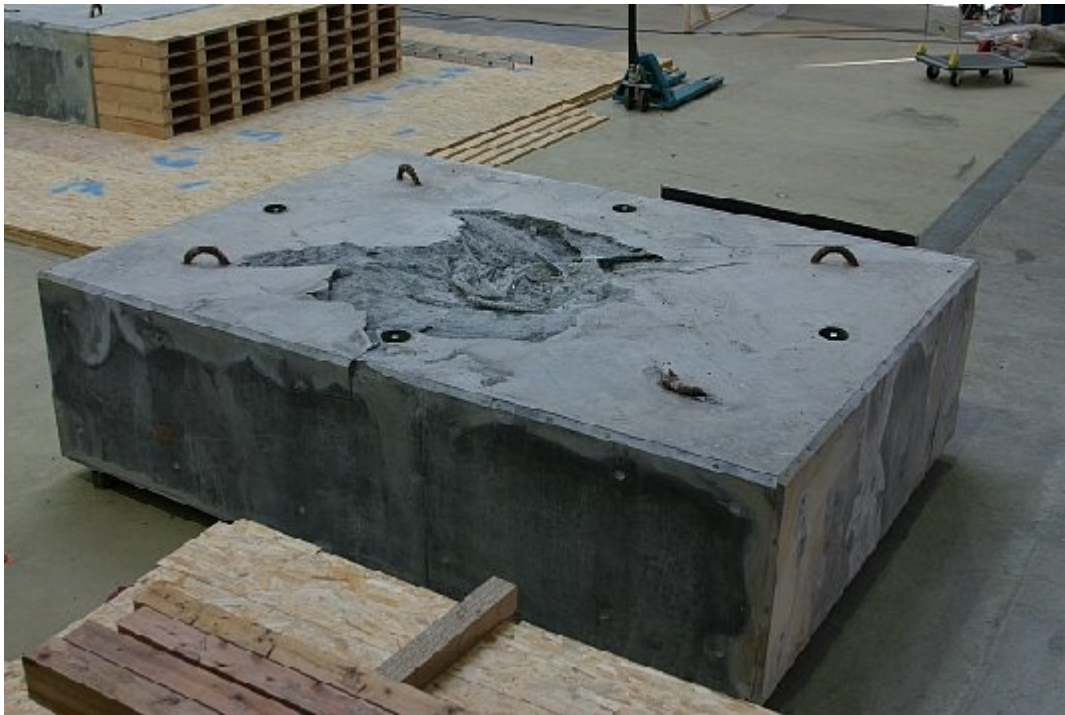
Figure 9: Disassembled and cleaned concrete target after the drop test with impact zone in the middle.
