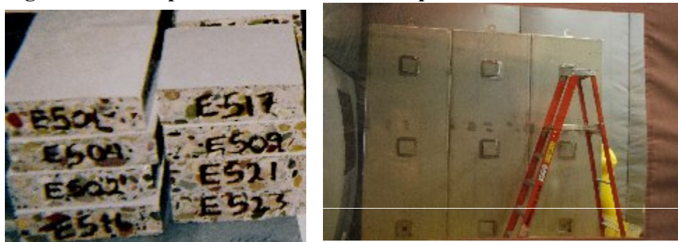
Figure 1. Close-up of Several Concrete Coupons and the Loaded Test Stand
