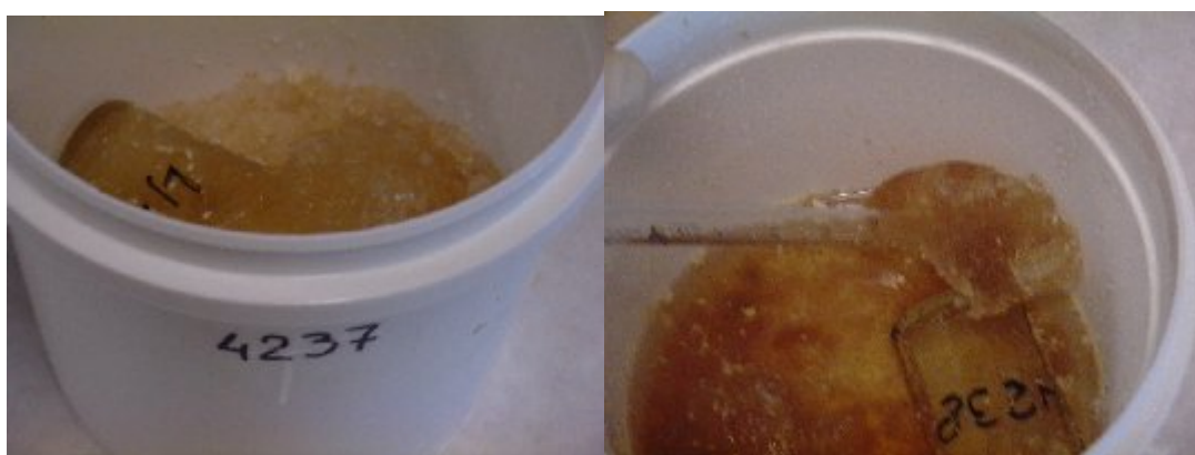
Fig. 2 Appearance of the specimen after solidification and after water has been added. (Low Level decontaminating solutions, # # 4237, 4238 in Table. 2.)
