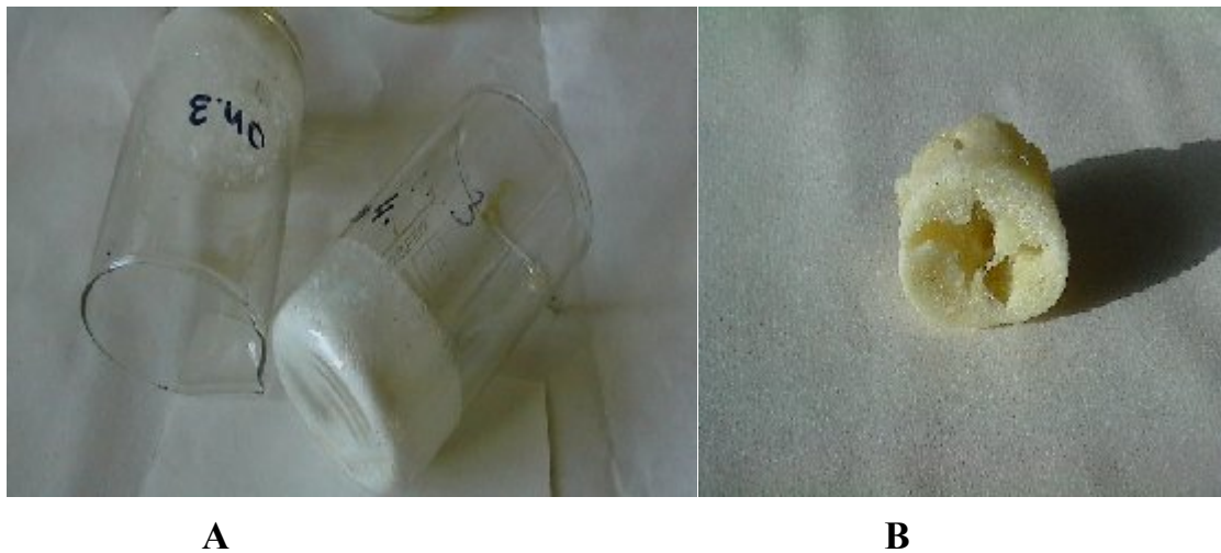
Fig. 1 (A) Appearance of specimen after solidification (B) After aging in air at room temperature
