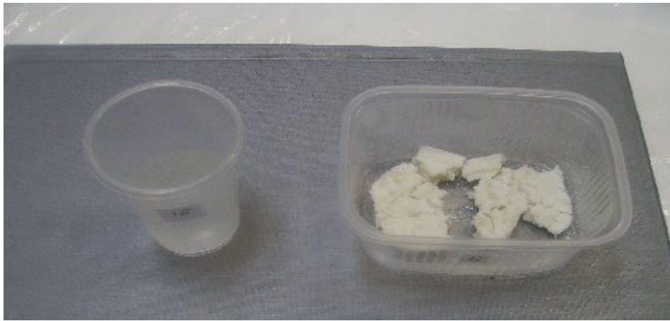
Fig. 3 The appearance of solidified specimen after water has been added. (Solution \text{HNO}_3 , 0,5M, # 15 in Table. 3.)
