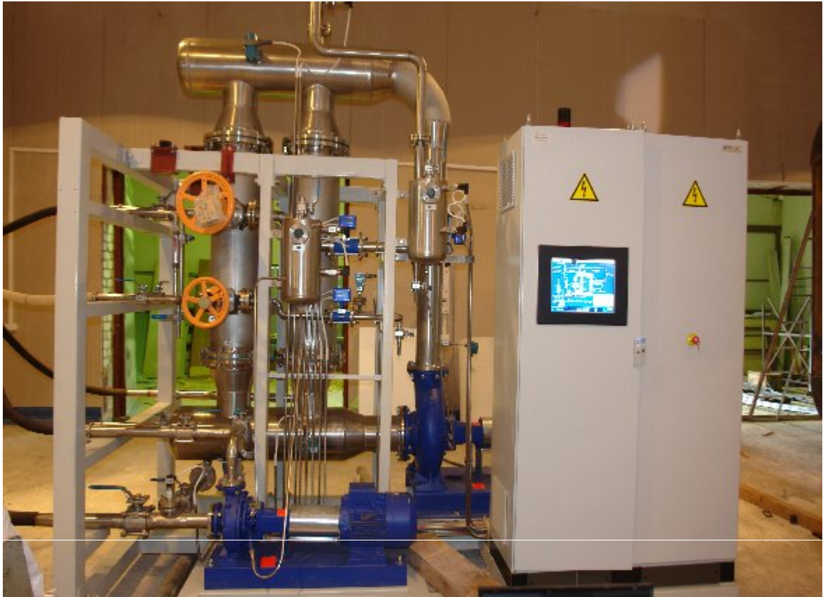
Fig. 4. Full-scale industrial prototype for concentrating suspended solids
