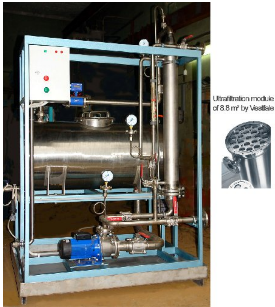
Fig. 3. Pilot ultrafiltration facility equipped with the tubular membrane filter cartridge module design
