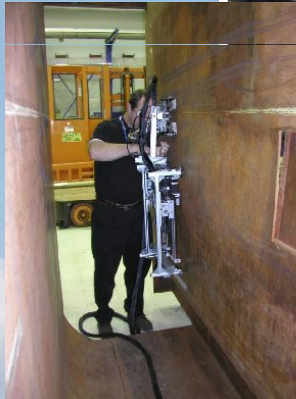
Left: Demonstration of Ultrasonic testing on Double-Shell Tanks
