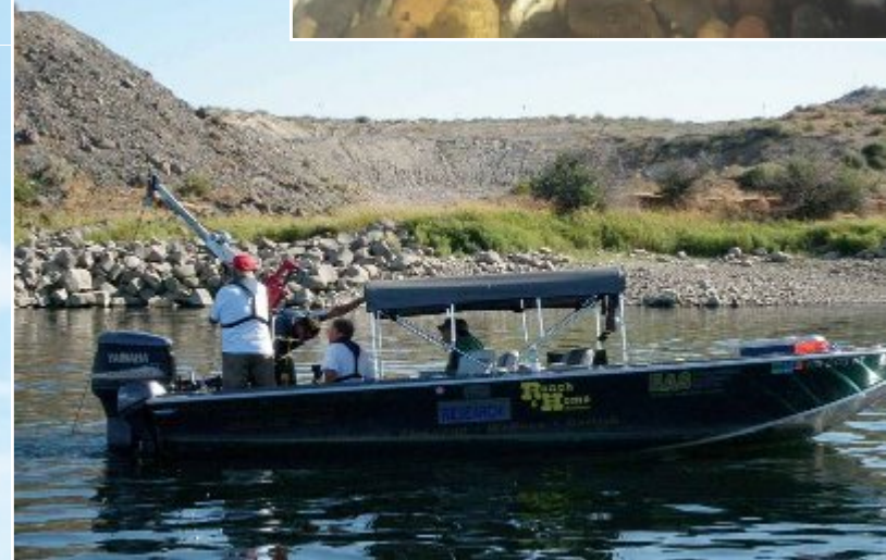
The Trident probe measures water temperature and conductivity
