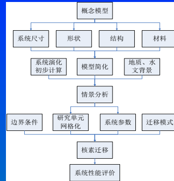
基于 Porflow 的性能评价流程图 Flowchart of Performance Assessment Based on Porflow Software
