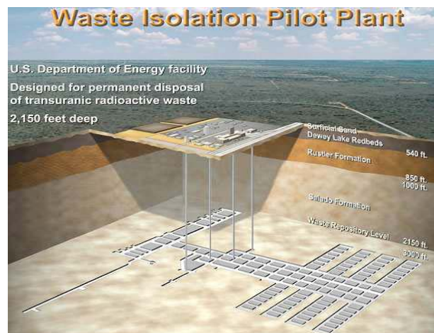
Fig. 4. The Waste Isolation Pilot Plant (WIPP), the only operating deep geologic nuclear waste repository, is excavated 700 meters below the surface in the massive salt of the Salado Formation, and has operated successfully since 1999.
