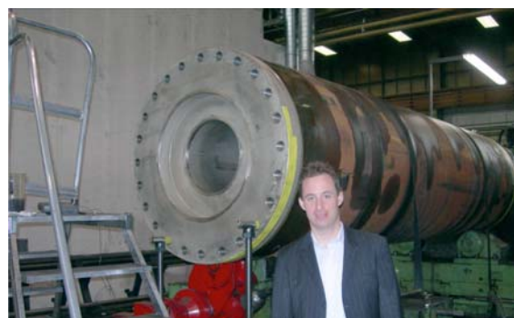
Fig. 15. Transfer cask during manufacturing
