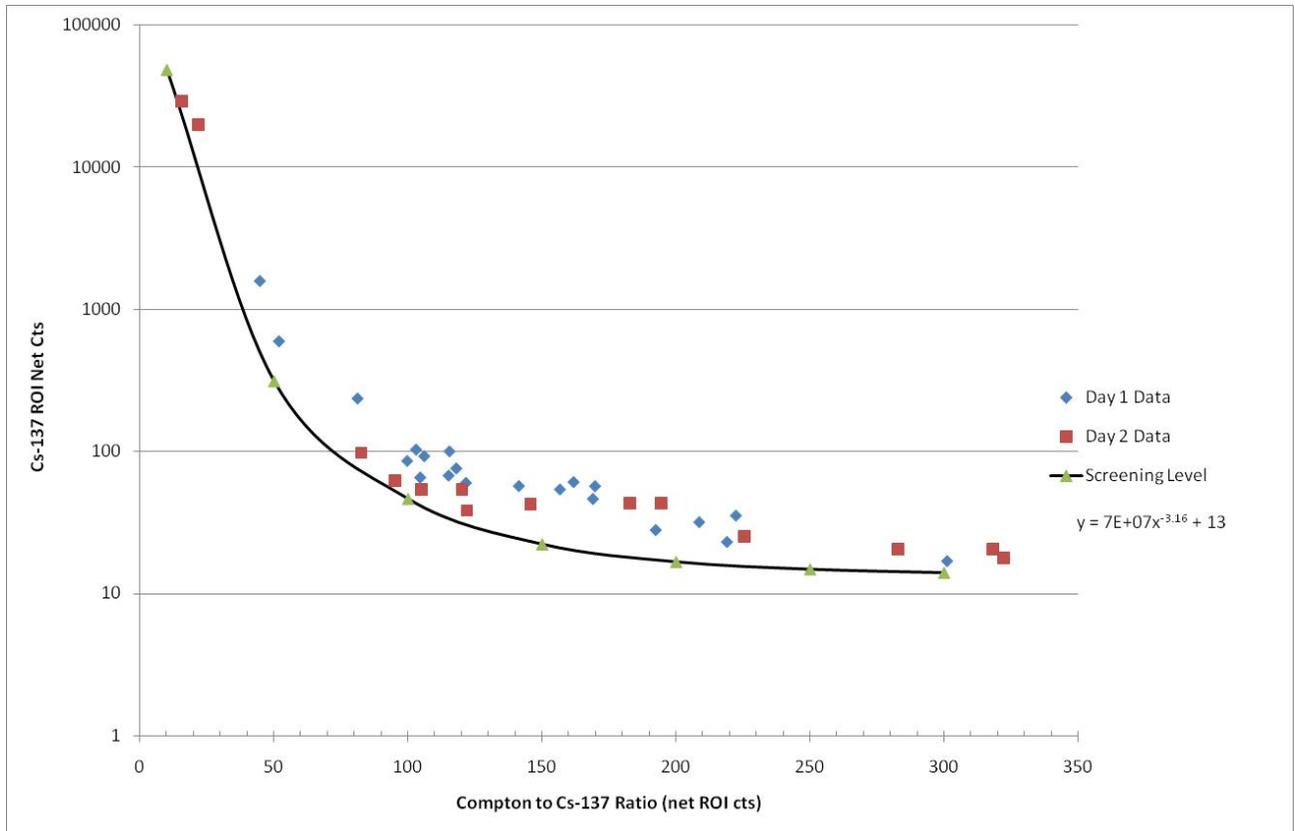
**Fig. 6. 1X1 Inch NaI(Tl) – Screening Level Compared with Field Measurements (adjusted to 4.1E+07 Bq Cs-137 SNF Fragment)**
