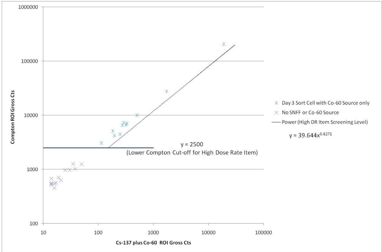
**Fig. 10. 1X1 Inch NaI(Tl) – Compton ROI versus Cs-137 + Co-60 ROI Gross Counts for Measurement with 5 mSv/h Co-60 Source in Excavator Bucket Compared with Bucket Measurements with no SNF Fragment or Co-60 Source**
