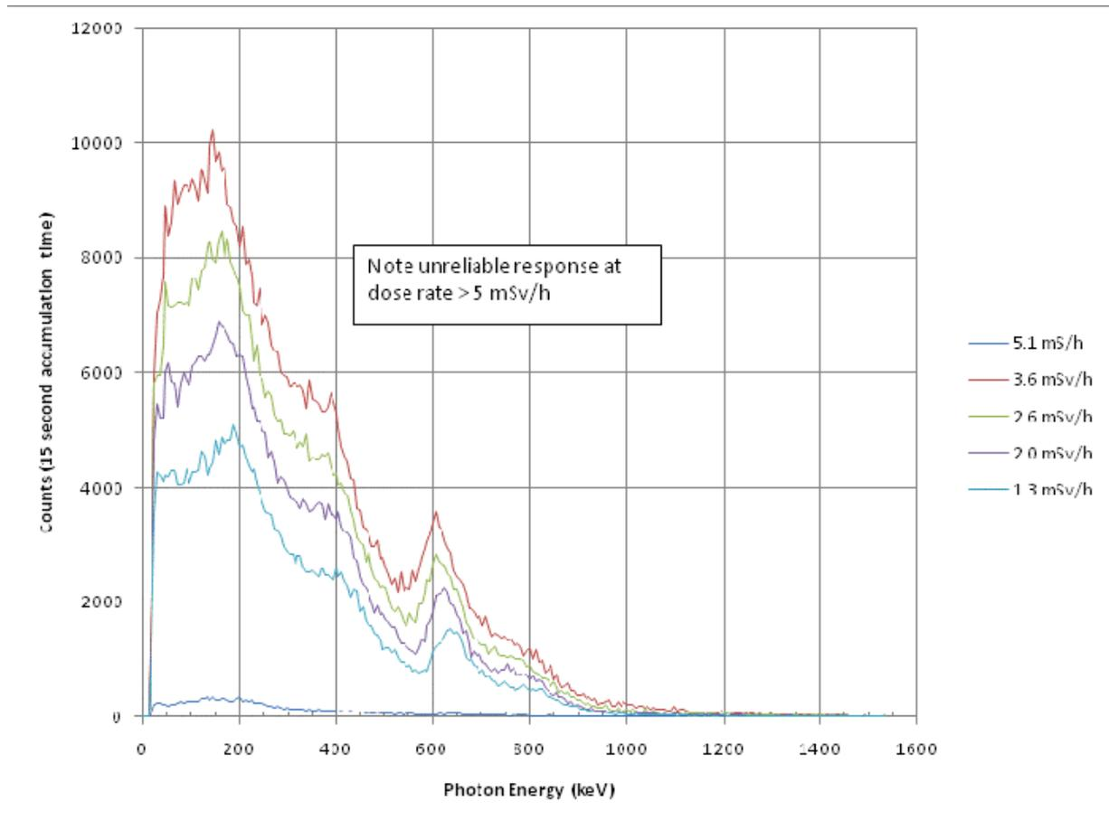
**Fig. 2. 0.25X1-Inch NaI(Tl) Detector Response as Function of Dose rate from a Cs-137 Source**
