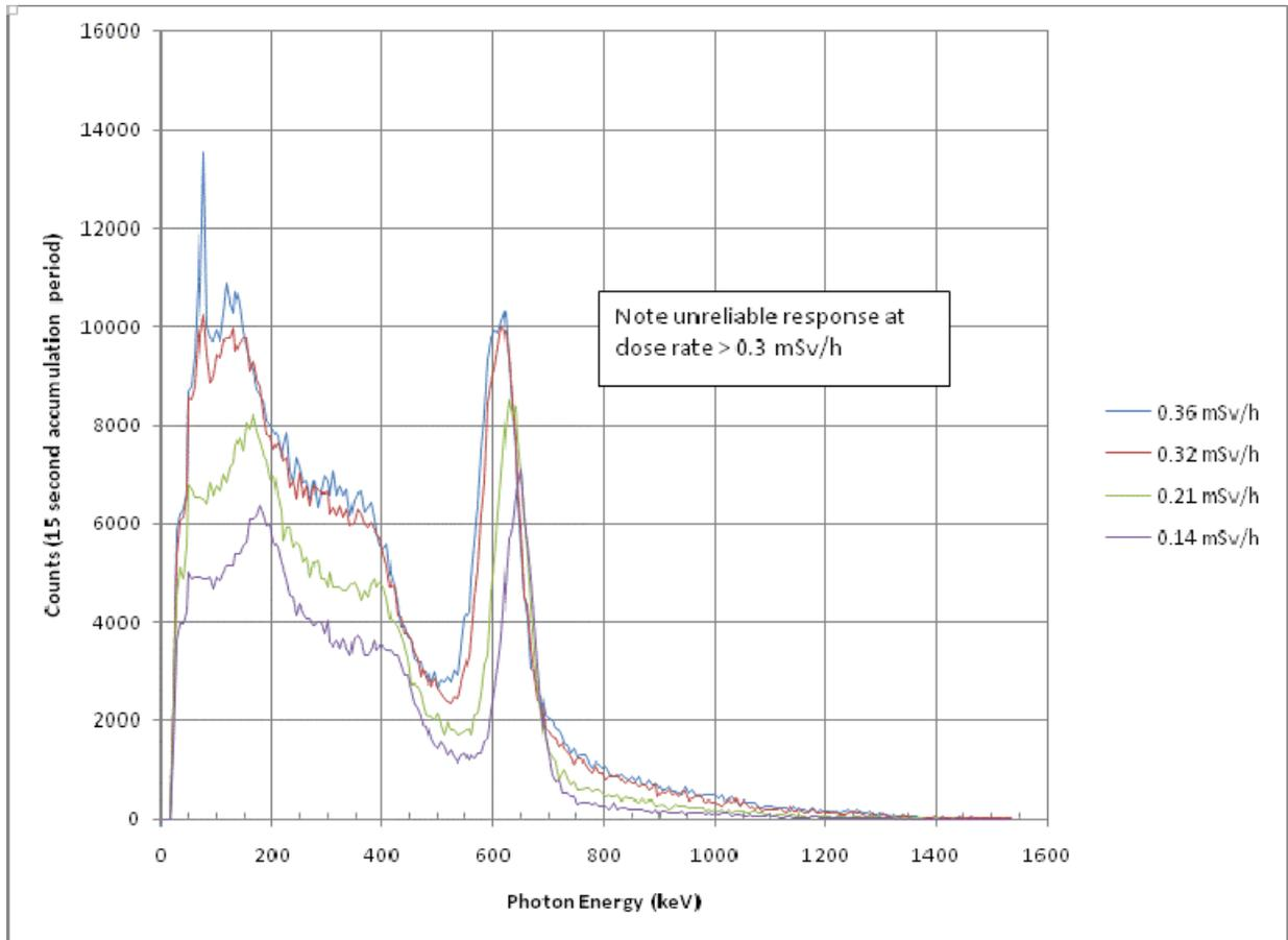
**Fig. 1. 1X1-Inch NaI(Tl) Detector Response as Function of Dose rate from a Cs-137 Source**
