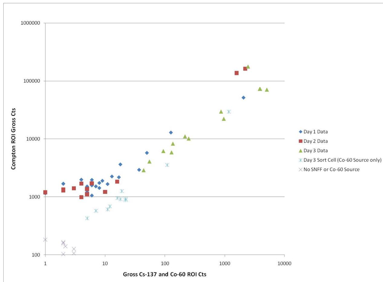
**Fig. 5. 0.25X1 Inch NaI(Tl) – Compton ROI versus Cs-137 plus Co-60 Gross Counts**
