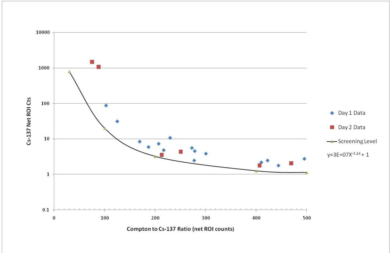
**Fig. 7. 0.25X1 Inch NaI(Tl) – Screening Level Compared with Field Measurements (adjusted to 4.1E+07 Bq Cs-137 SNF Fragment)**
