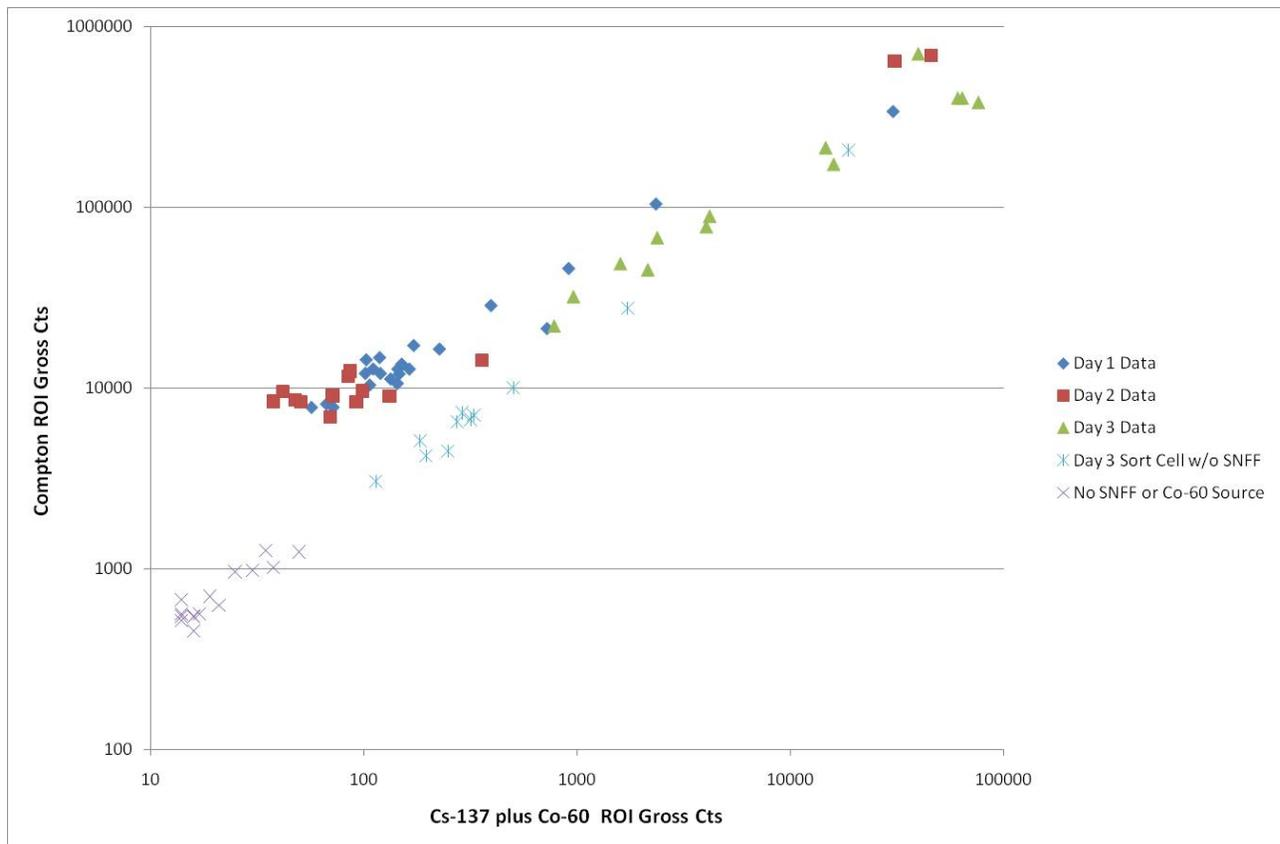
Fig. 4. 1X1 Inch NaI(Tl) – Compton ROI versus Cs-137 plus Co-60 Gross Counts
