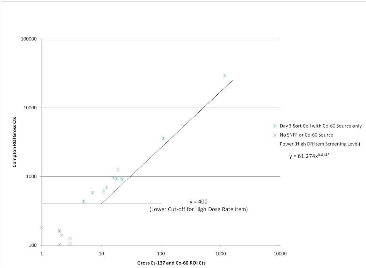
**Fig. 11. 0.25X1 Inch NaI(Tl) – Compton ROI versus Cs-137 + Co-60 ROI Gross Counts for Measurement with 5 mSv/h Co-60 Source in Excavator Bucket Compared with Bucket Measurements with no SNF Fragment or Co-60 Source**
