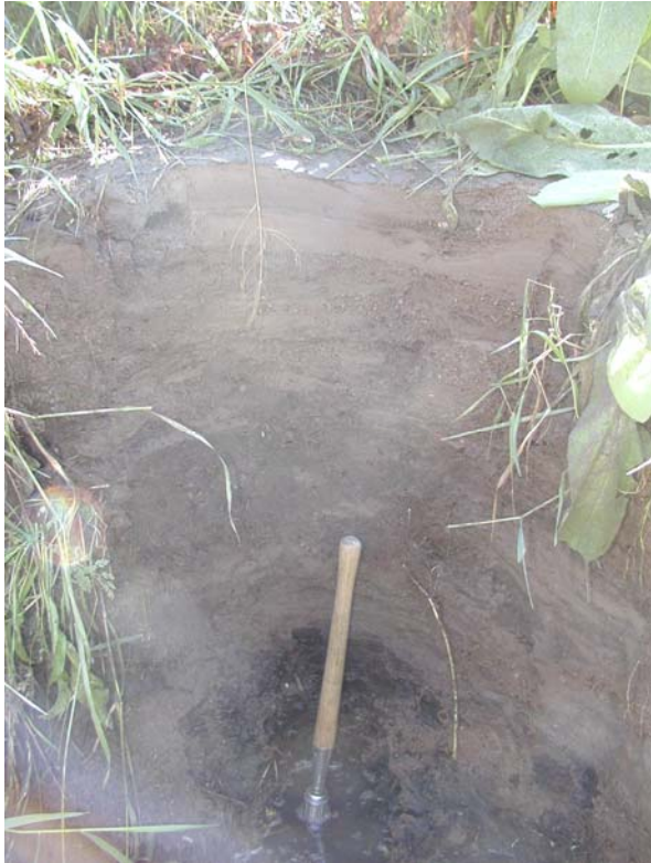
Figure 2 (a) Photograph of headcut and eroded channel within the Pueblo Canyon wetland and (b) photograph of approximately 1 meter of post-fire sediment aggradation resulting from trapping efficiency in stable, vegetated portions of wetland. Dark ash-rich sediment layer is visible at base of excavation.
