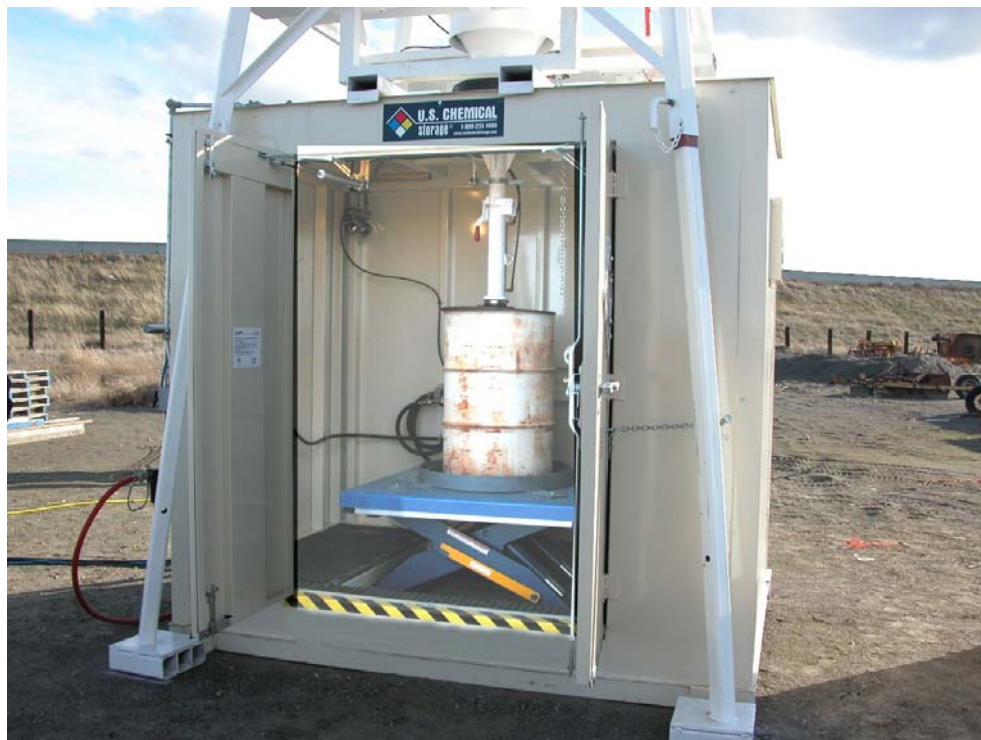
Fig. 3. Drum penetrating facility used to open and sample drums and bottles.
