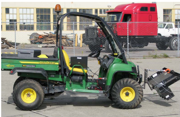
Fig. 2. CABRERA Large Area Scanning System (CLASS) Front-Mounted on ATV
