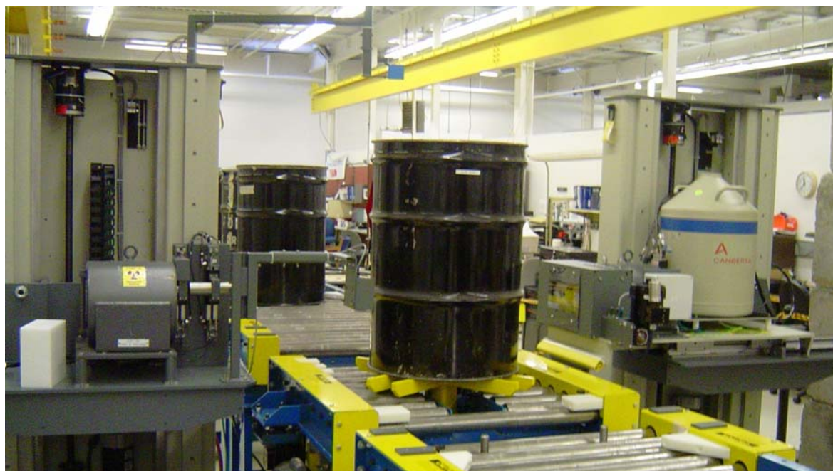
Figure 1. Photograph of the TGS system during factory assembly. The transmission assembly is viewable on the left and the beam modulator and shutter mechanisms are visible. To the right is the germanium detector and surrounding aperture box. The drum is shown on the translation assembly in the raised position of the rotator above the roller conveyor.
