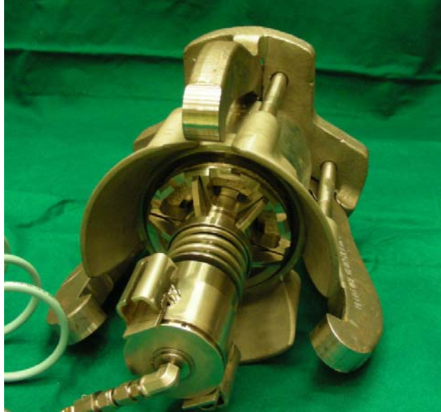
Fig. 8. Installation Tool in Hanford Connector
