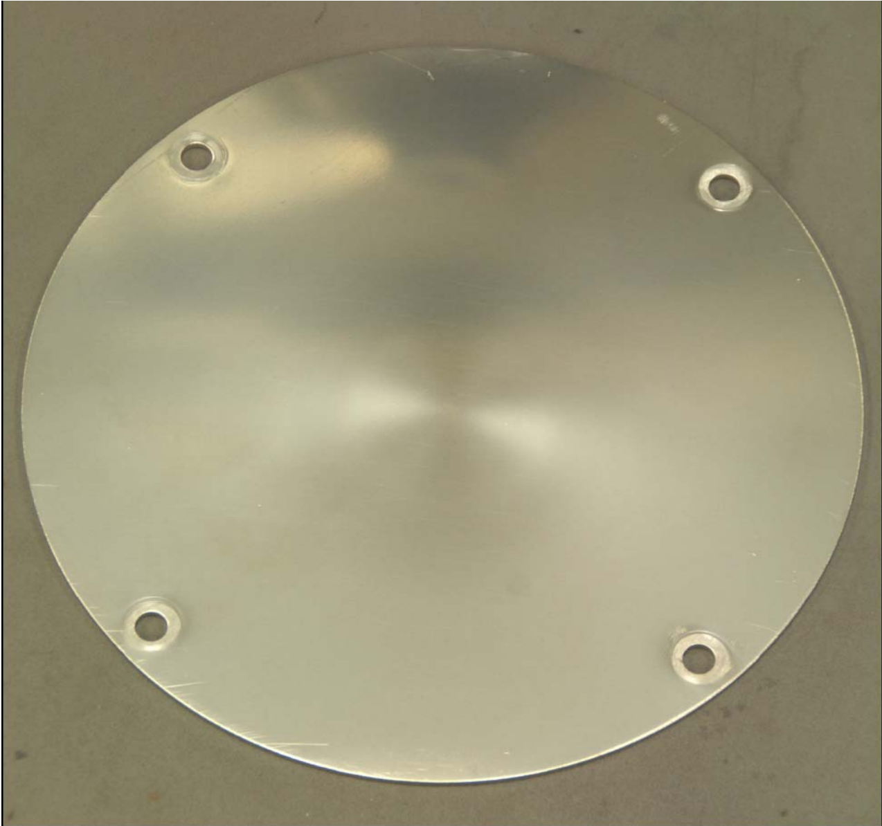
Fig. 3. Test coupon after 96 hours of erosion
