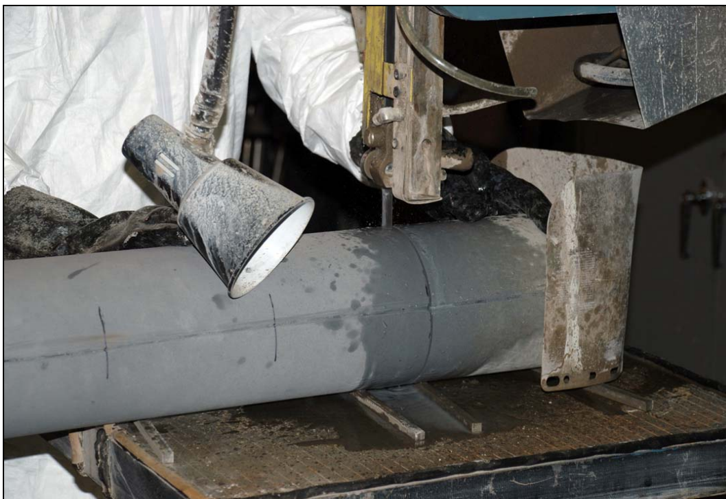
Figure 3. Gamma Guard II and Portland cement column sample being cut into sections.
