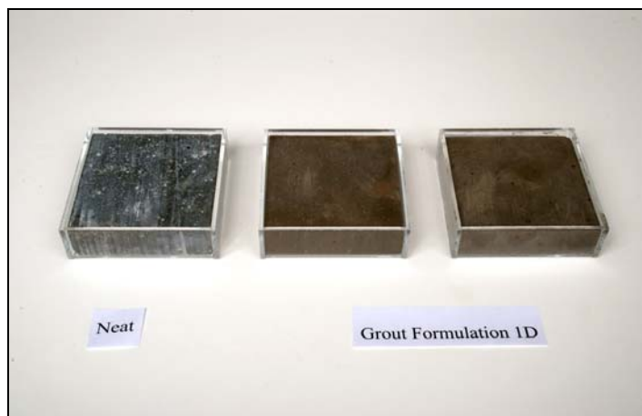
Figure 1. Grouted samples generated using Gamma Guard I and Portland cement and the neat Portland cement sample.
