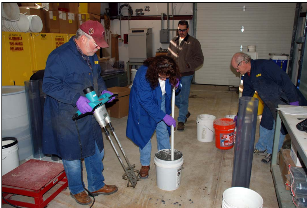
Figure 2. Gamma Guard II and Portland cement sample during the mixing process.
