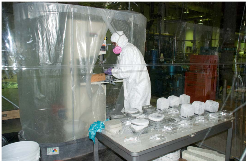
Fig. 4. Rainwater and Aqueous Organic and GG II samples solidified with Portland cement during the cutting process.
