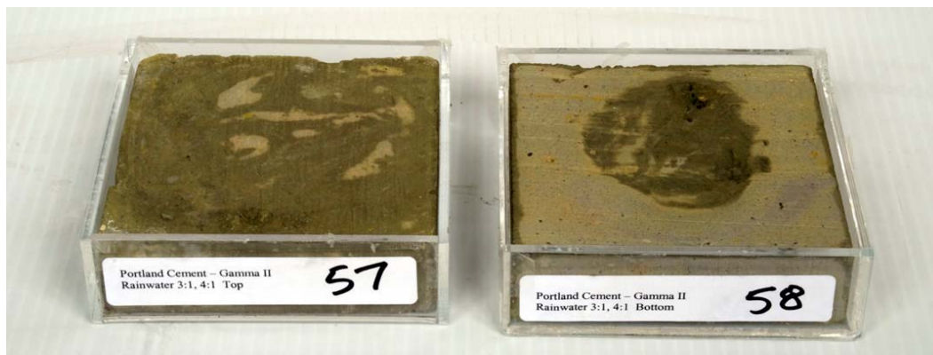
Fig. 3. Sample 58 shows the melted metal smear of the shielding material.
