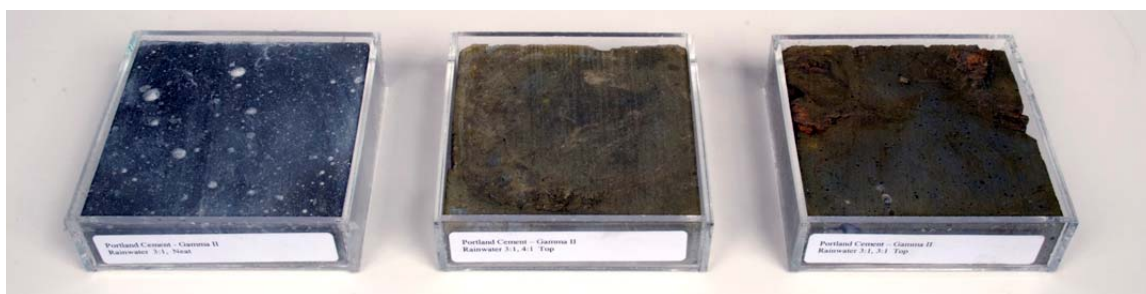
Fig. 2. The Rainwater Portland cement 3:1 neat sample (left) and the top sample sections for the 3:1 to 3:1 shielded sample (middle) and the 3:1 to 4:1 shielded sample (right).
