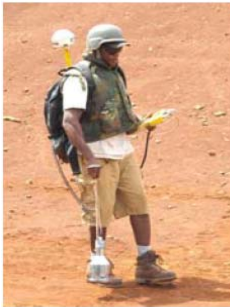
Fig. 1. Typical GWS in UXO area with Technician Wearing Flack Vest and Helmet
