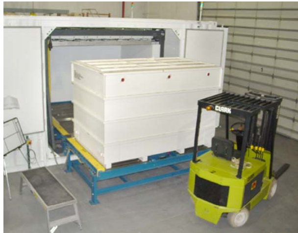
Fig.1. Box Neutron Assay System (shown with SLB-2 on the load conveyor).
