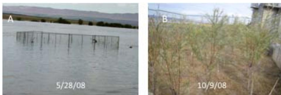
**Fig. 6. Sr-90 phytoextraction using Coyote willows. Pictures of treatability test plot during second year of growth: a) picture taken 5/28/08 showing natural spring flooding of site; b) trees just before second-year harvest on 10/9/08.**
