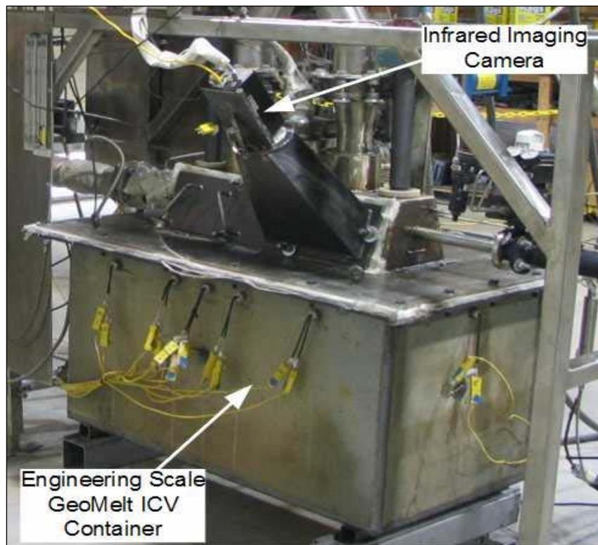
**Fig. 3. Engineering-scale GeoMelt ICV melter and position of infrared camera.**
