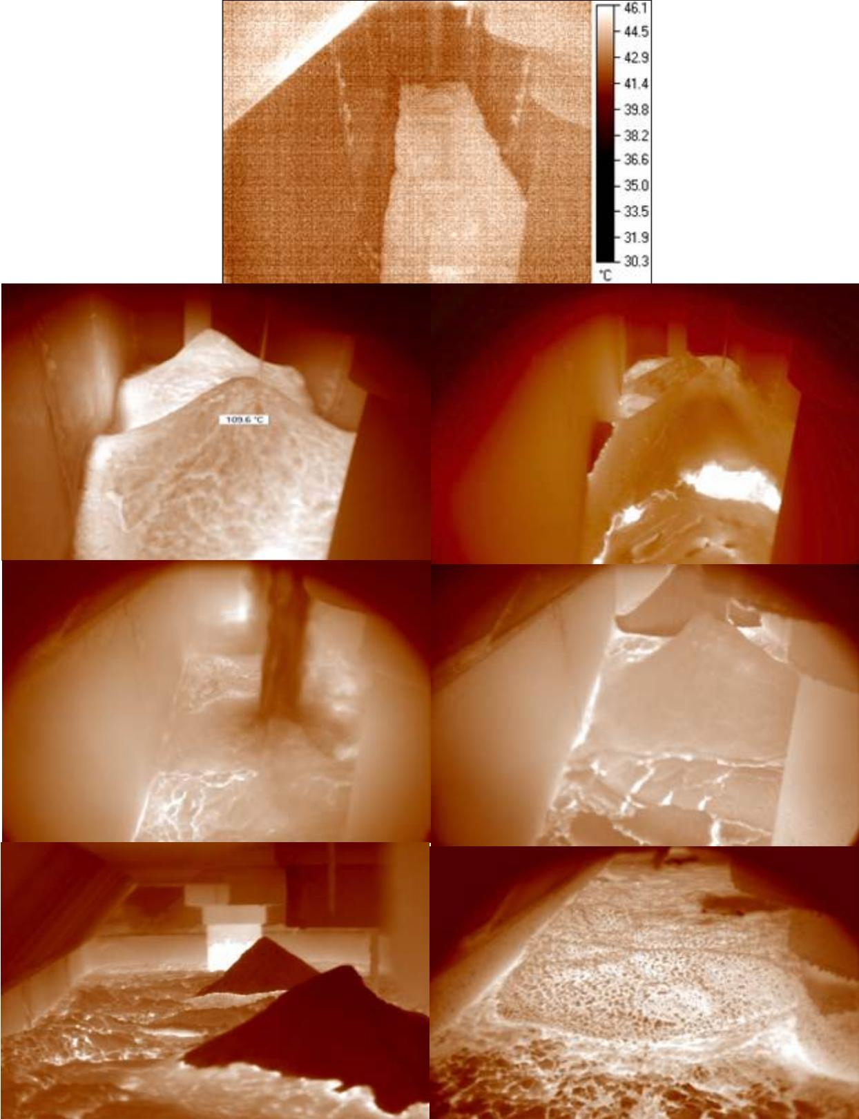
Fig. 4. Still images of DBVS ICV container using a thermal imaging system.
