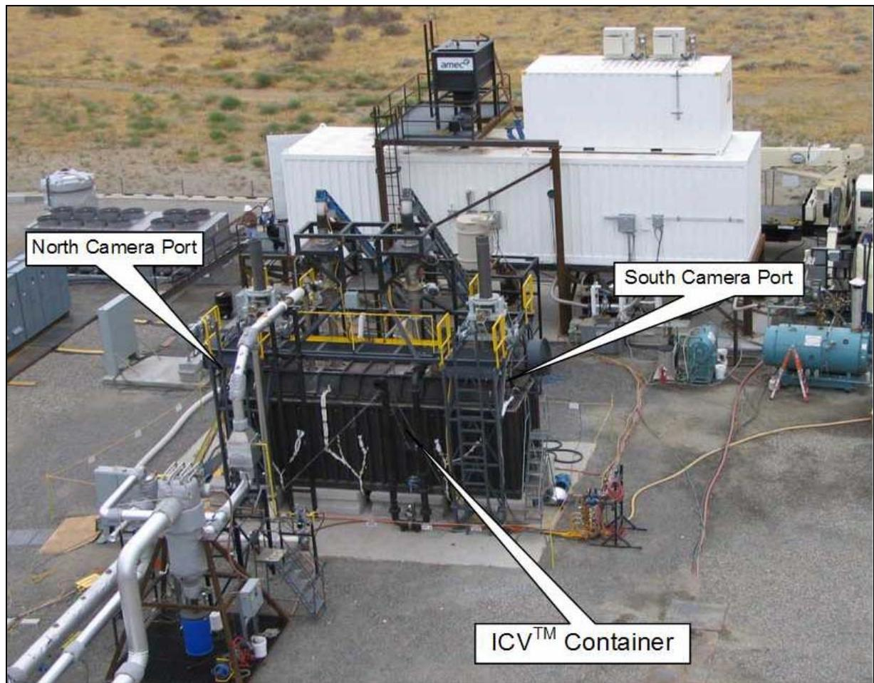
**Fig. 1. View of GeoMelt ICV Container and Camera Port Locations**
