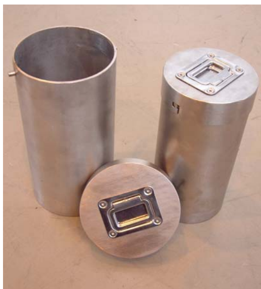
Fig. 4. Photograph of one of the mock 3013 containers used. The inner can is shown to the right of the unlidded outer can.
