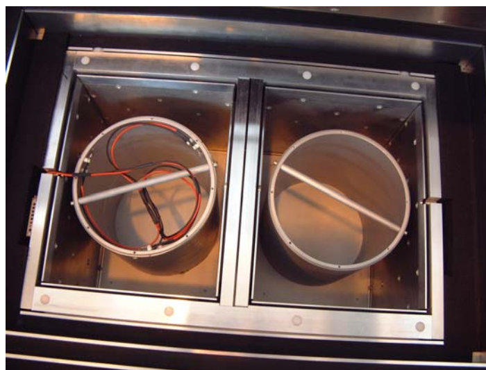
Fig. 2. Photograph of the Joule effect heater (left) and dummy (right) inside the calorimeter. The power cable exits through the notch.
