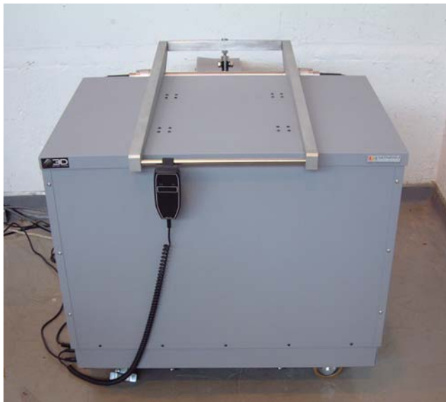
Fig. 1. In-situ photograph of the Calo Series 270 calorimeter used.
