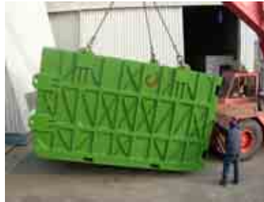
Figure 4. Four m long, 3 m wide metal extracted structure storage box during transport.
