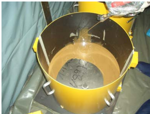
Fig. 16: grouting of a pellet
