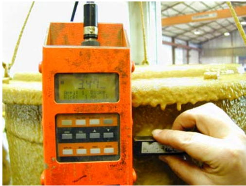
Fig. 4: Coat thickness measuring
