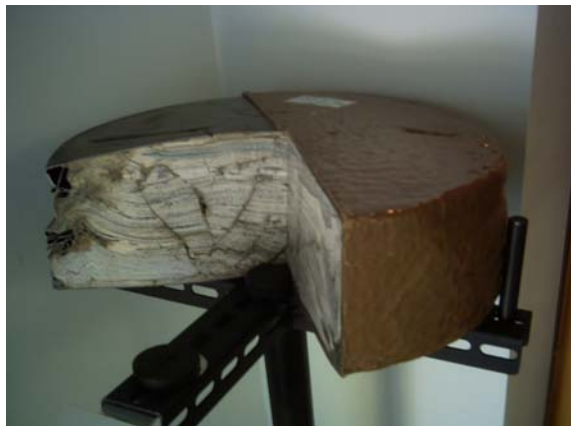
Fig. 14. pellet half coated with polyurethane
