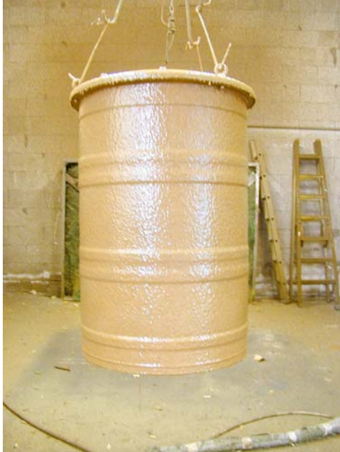
Fig. 3: Polyurethane coated barrel
