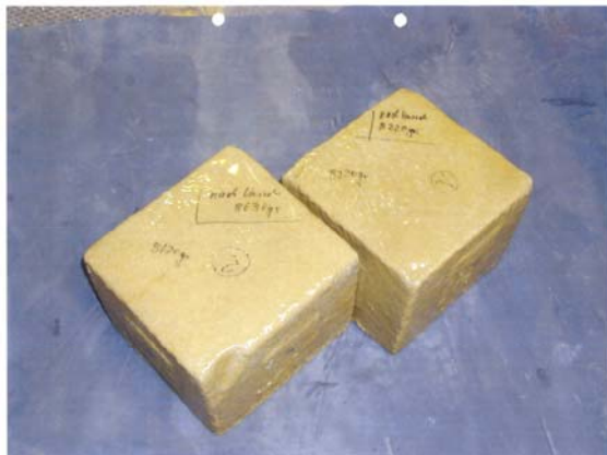
Fig. 13: Coated and weighted Ytong stones
