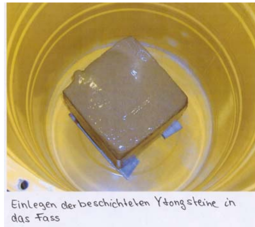
Fig. 12: Ytong Stone in the drum
