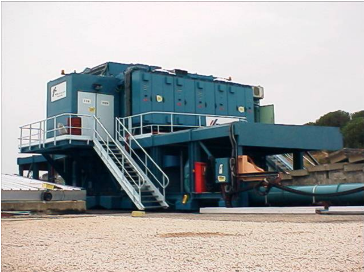
Fig. 1. Photograph of AREVA's first-generation mobile hot cell (ERFB) deployed at the Marcoule Site, France.
