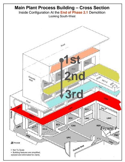
vessels and piping is enabled because the Inside-Out Demolition Plan does not require any prior surface decontamination (e.g., scabbling, scarifying, pressure spray) of walls, floors, and ceilings. In fact the MEOSI dose is minimized in the Inside-Out Demolition by avoiding surface decontamination. The contamination is left in place and fixed to the surface, thus minimizing the generation of airborne contamination during demolition.
