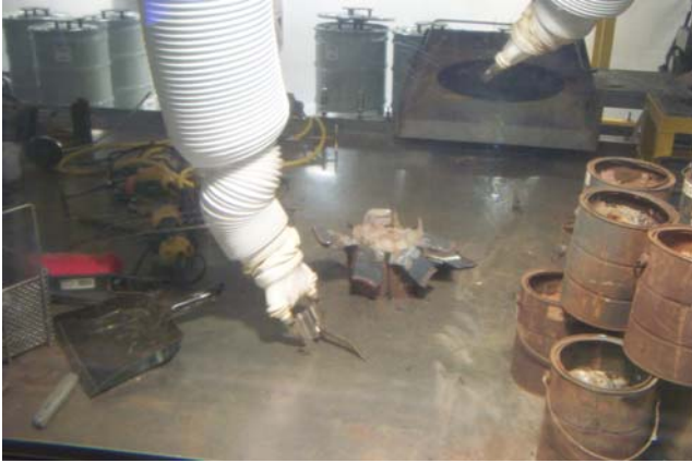
Fig. 8, Paint Can with Poly in Hot Cell
