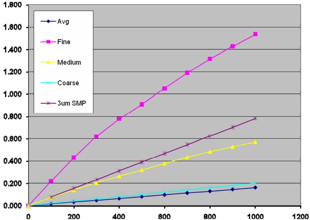
Fig. 5. Differential pressure vs. flow rates for standard vs. membrane filters.
