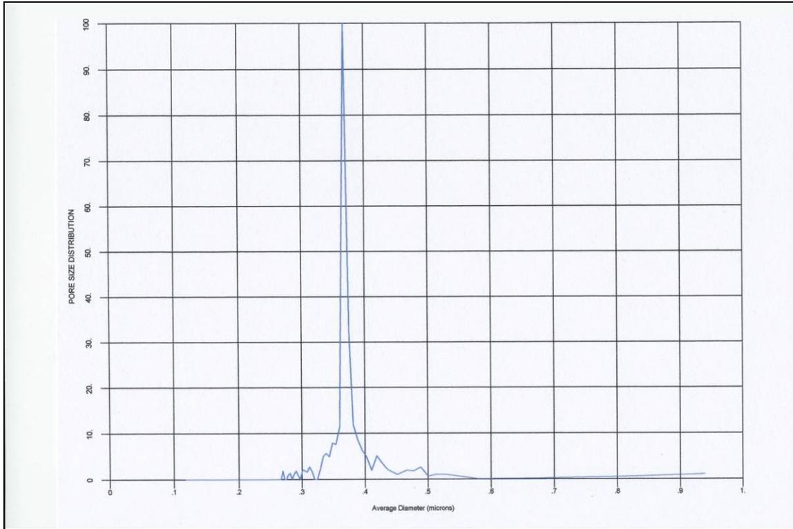
**Fig. 3. Pore size and pore size distribution as measured by porometry.**
