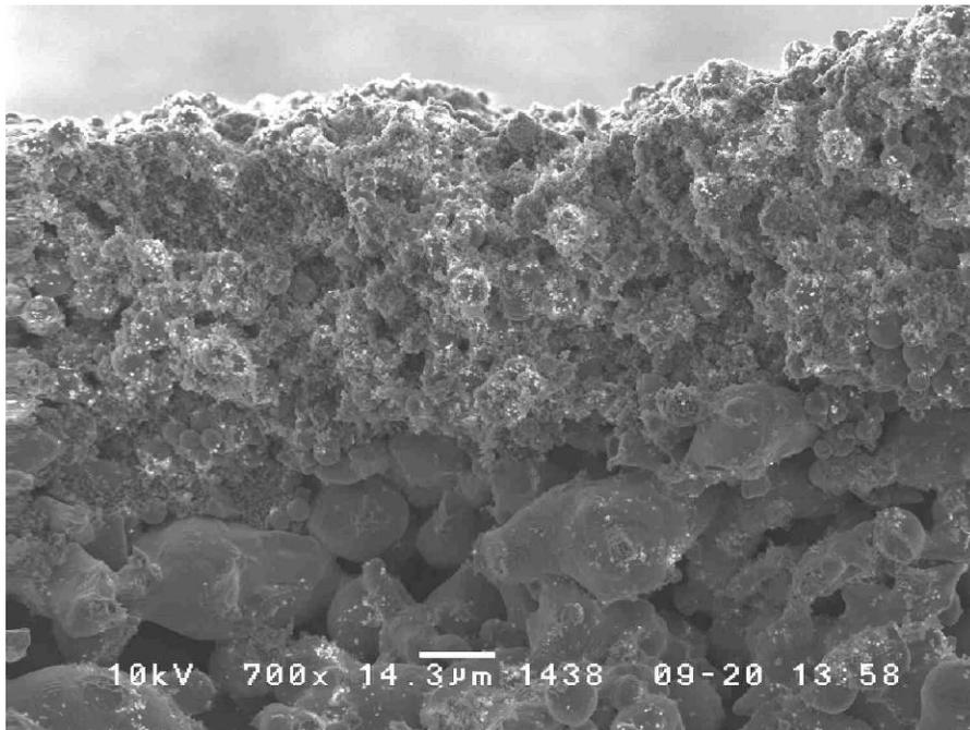
**Fig. 1. SEM image of fractured membrane showing the sintered powder interface.**
