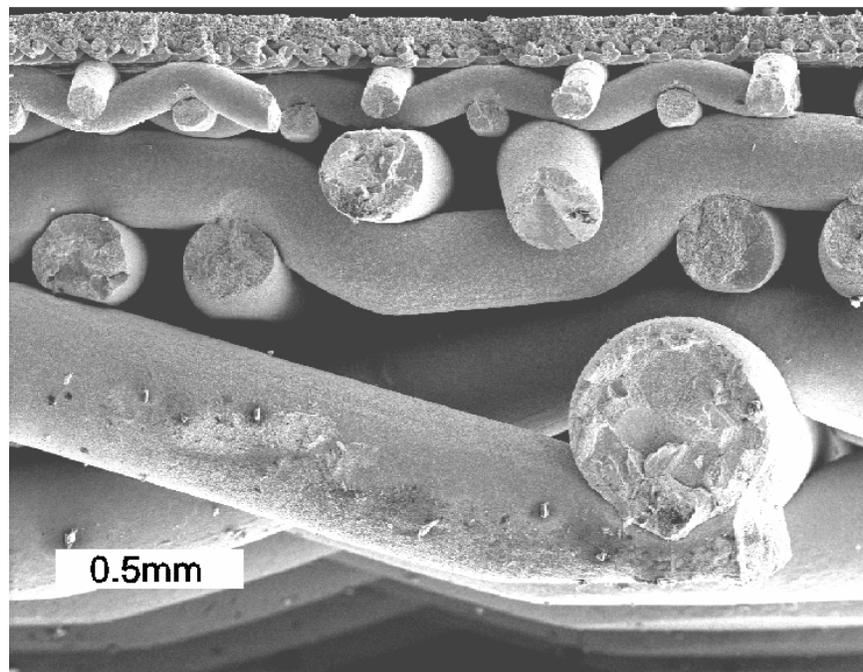
**Fig. 2 SEM image of a fractured membrane showing the sintered wire mesh interface.**
