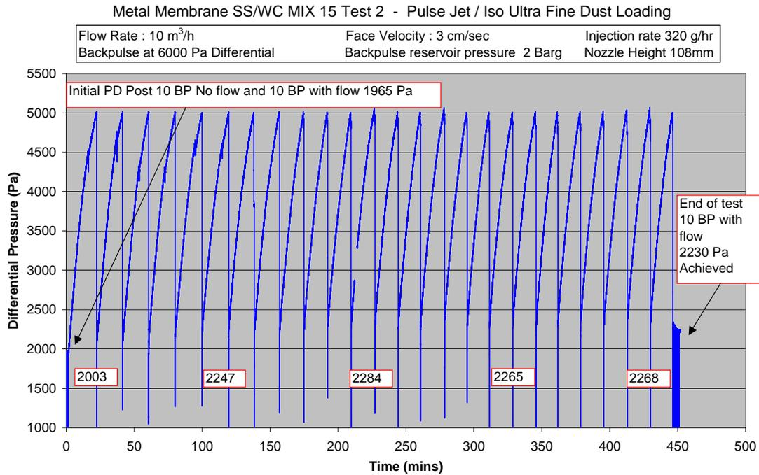
**Fig. 4. Blow-back chart for filter cleaning showing back-pulsing for removal of ultra-fine dust.**
