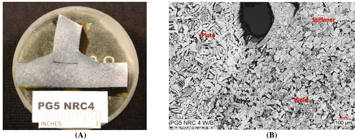
Fig. 7. Metallurgical specimen from Sample NRC 4 after mounting, polishing, and etching (A). Microstructure of stiffener fillet weld, plate girder, and stiffener (B).
