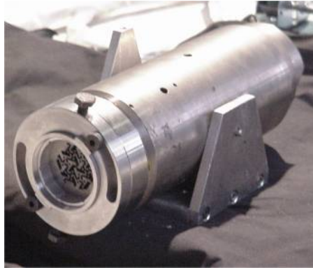
Fig. 2. Aladin II in coded aperture mask configuration
