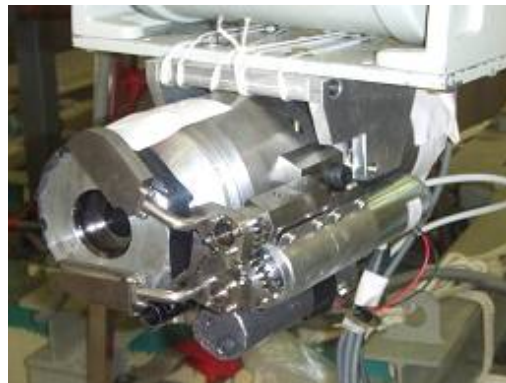
Fig. 6. Antipinhole collimator on a gamma camera
