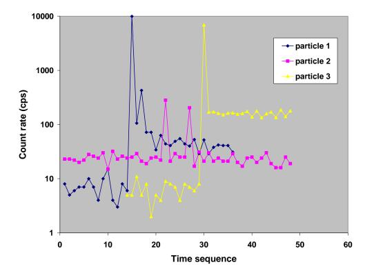
Figure 5. Profiles of count rate obtained by a detector placed near the entry port of particle receipt tank on the ROV. These three particles were retrieved at various times during surveys on 25 September 2008.
