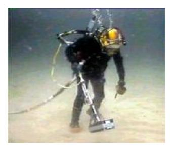
Figure 1. Diver surveying seabed using improved plastic scintillation detector at the end of an ergonomically designed crutch.
