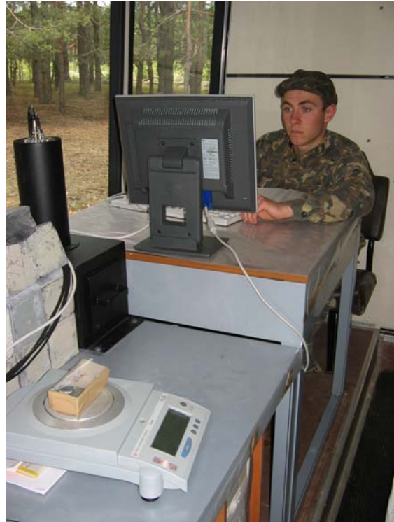
Figure 3. IRL staff member measuring Cs-137 and Sr-90 concentrations in birds in a mobile laboratory
