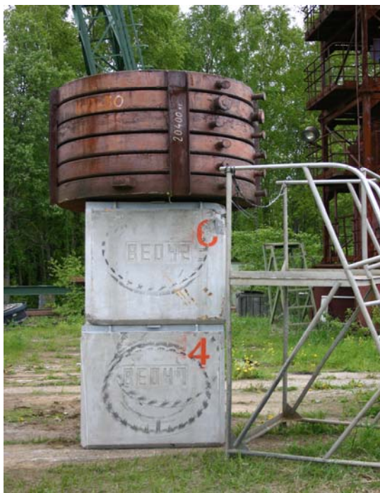
Fig. 1. Mechanical tests for containers with cemented wastes.
