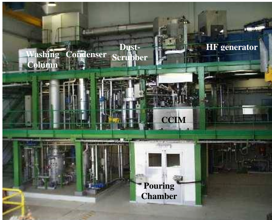
Fig. 1. General view of the 650 mm diameter CCIM demonstration platform – CEA Marcoule
