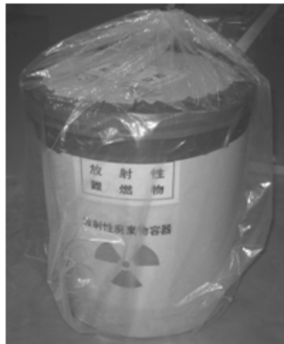
Fig.1. Waste package for plutonium contaminated wastes (20ℓ carton box)
