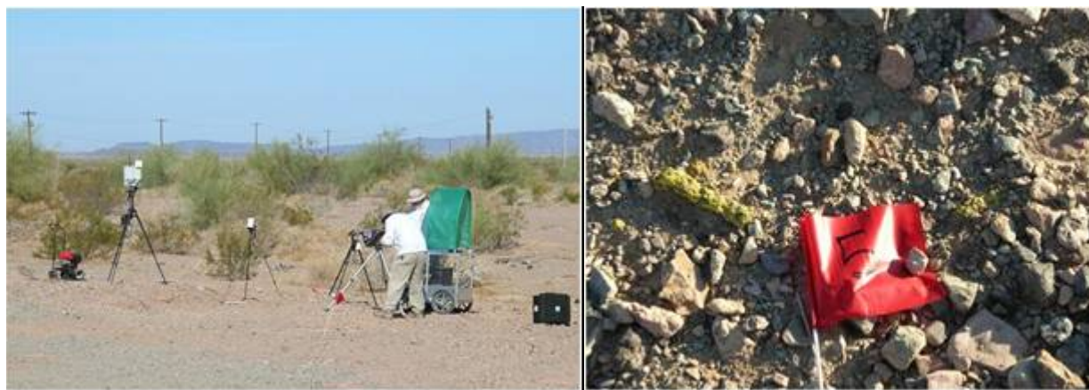
Figure 1. Left photograph shows image acquisition of fired DU penetrator by FSI and by other ICET imaging techniques near DU catch box at Yuma Proving Ground, AZ. Photograph on right shows two DU penetrators in situ ; a red plastic marker flag is included for identification.
