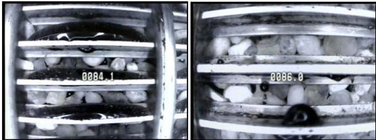
Figure 8. Down-well Photographs of Recovery Well Screens (100-slot) with Visible Creosote.
