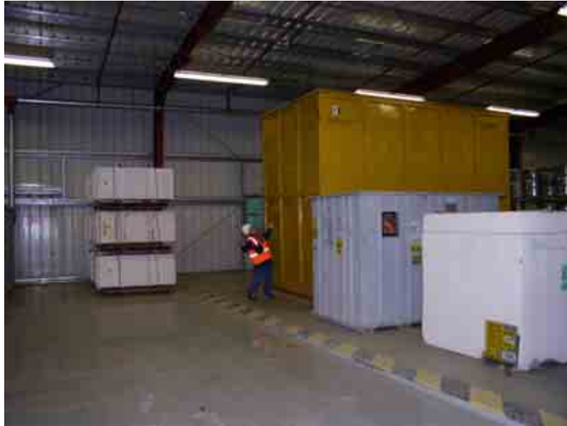
Fig. 1. Typical oversize waste container in storage.
