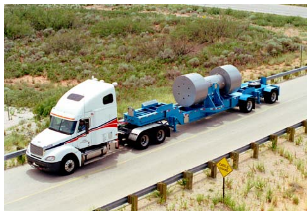
Fig. 4. Remote Handled nuclear waste ( >100 nanoCi/gram of waste but <23 Ci/liter), some of it from reprocessing of spent fuel, being transported to the WIPP site in New Mexico in a 72B cask.
