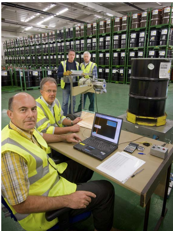
Figure 1 SNAP monitoring a waste drum on a turntable
