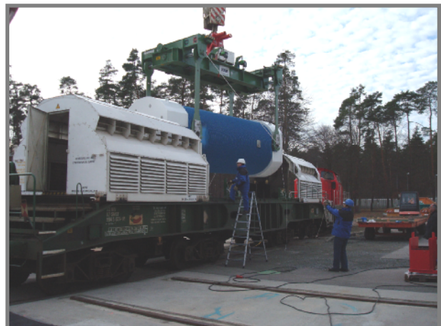
Fig. 5: Loading of the CASTOR cask on the train (test)
